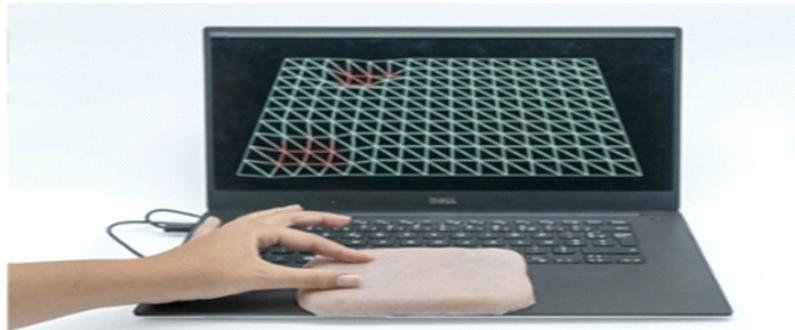
Researchers created a phone case, computer touch pad and smart watch to demonstrate how touch gestures can convey expressive messages for computer mediated communication
