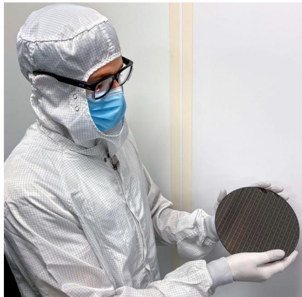
Dr. Alejandro Cortese, displaying a silicon-on-insulator wafer that contains finished CMOS “brains.”
